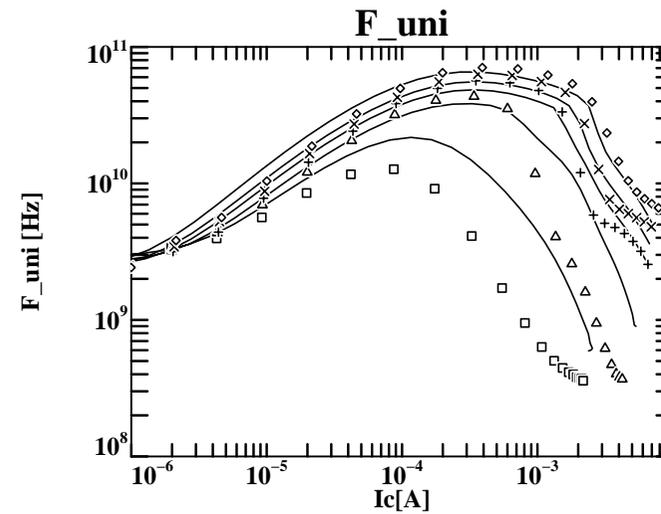
process E: NPN of a BiCMOS process
