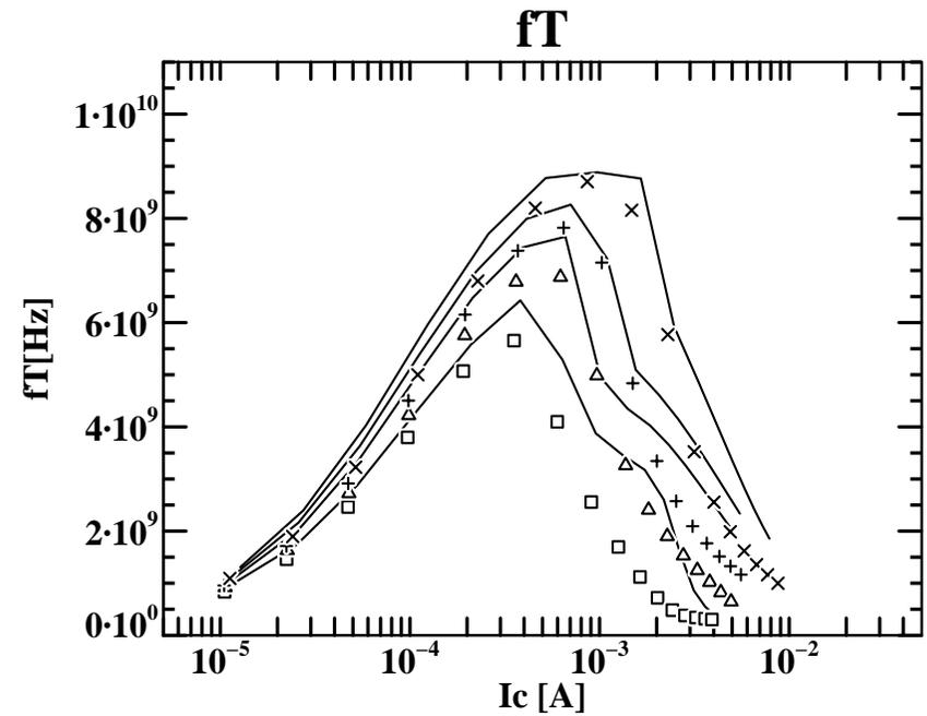
process D: NPN of a double poly BiCMOS process
