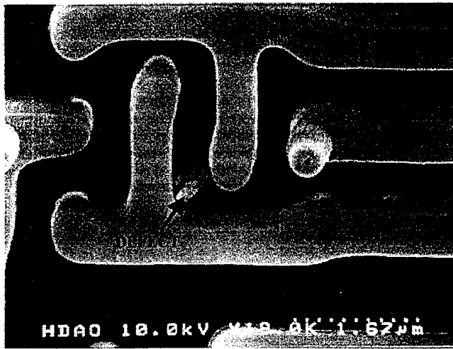
Fig. 20. Metal particulate contamination at metal one layer.
