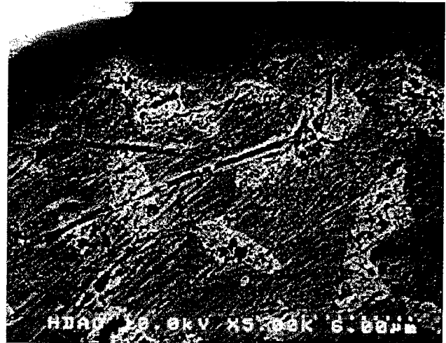
Fig. 52. SEM micrograph showing the intermetallic formation after high temperature assembly.
